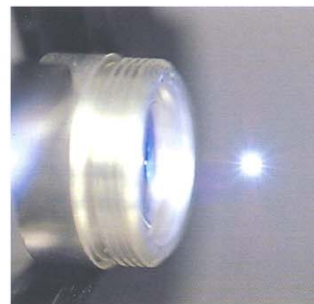
Figure 3 Breakdown in air by a microlaser with a pulse energy of 2.7 mJ. Optics allows greater freedom over the location of fuel ignition.
