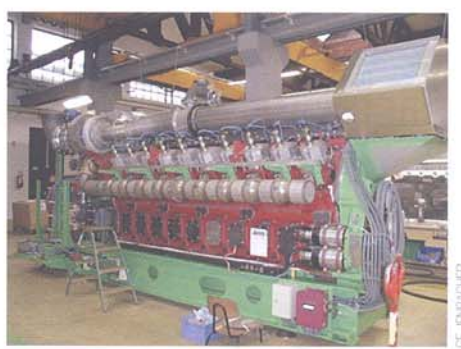
Figure 5 Application of laser ignition in an industrial gas engine.
