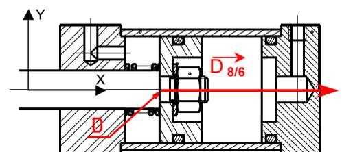
$$\{\mathcal{T}_{8/6}\}_D = \left\{ \begin{matrix} \vec{D}_{8/6} \\ \vec{M}_{D(8/6)} \end{matrix} \right\}_D = \left\{ \begin{matrix} X_{8/6} & 0 \\ 0 & 0 \\ 0 & 0 \end{matrix} \right\}_{(\bar{x}, \bar{y}, \bar{z})}$$
